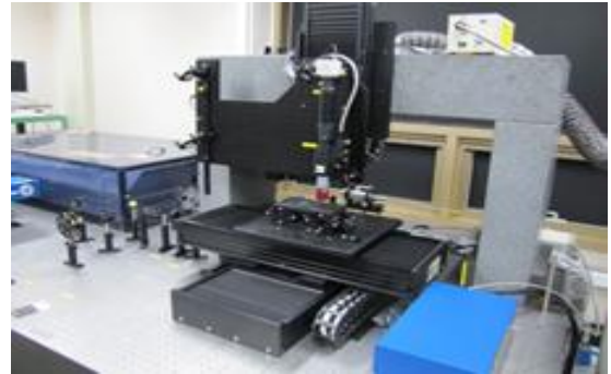
Fig. 1 Image of ultrafst laser machining processing system
