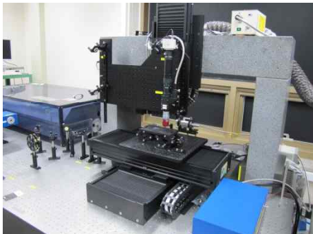
Fig. 1 Image of laser processing system
