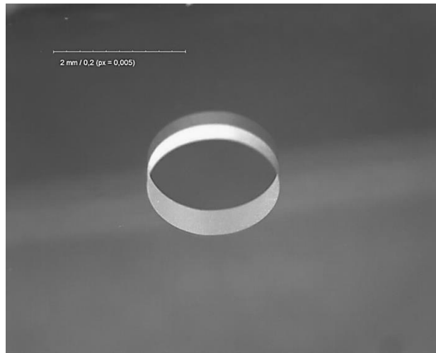
2 mm dia. hole in 0.55 mm thick non-strengthened aluminosilicate glass, v = 100 mm/s
