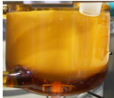
end of reaction: strong scattering due to microgel particles
