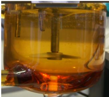
start of reaction: no particles; monomers in solution
