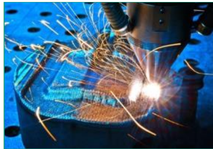
Laser cladding process
