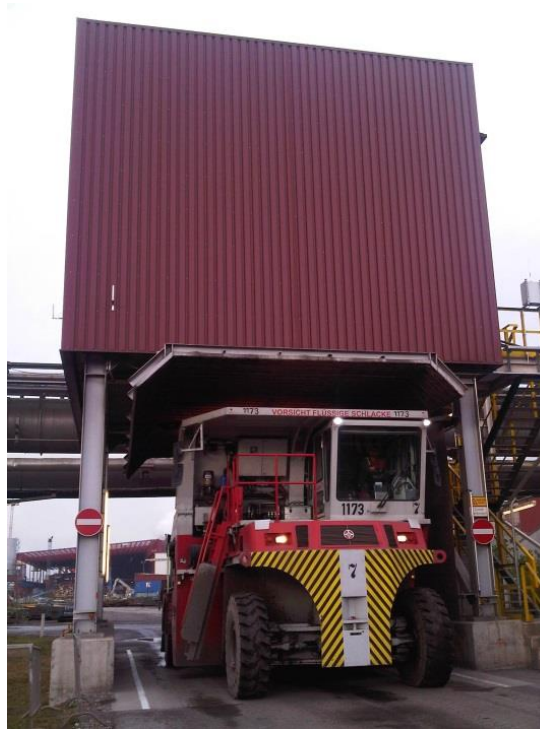
slag transporter underneath measuring cabinet
